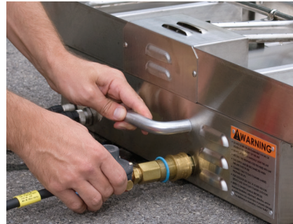
FIGURE 5: PROPANE HOSE QUICK DISCONNECT OUTLET
